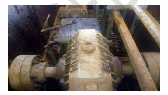
Fig 2.12 Intake gate hoisting system
